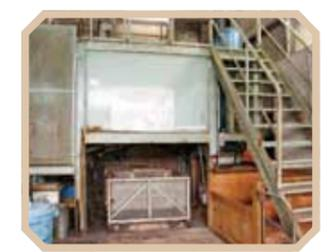
Kitchen waste is inserted from the top of this machine where it is fermented for three hours.
