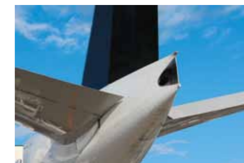
Exhaust port of an auxiliary power unit (APU)
