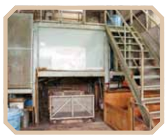
Kitchen waste is inserted from the top of this machine where it is fermented for three hours.
